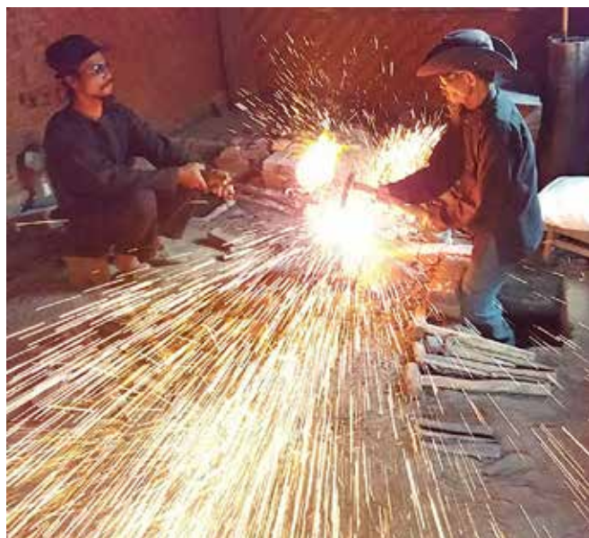
Sparks fly when forging layers of iron and nickel. Photo by Nick Kasten
