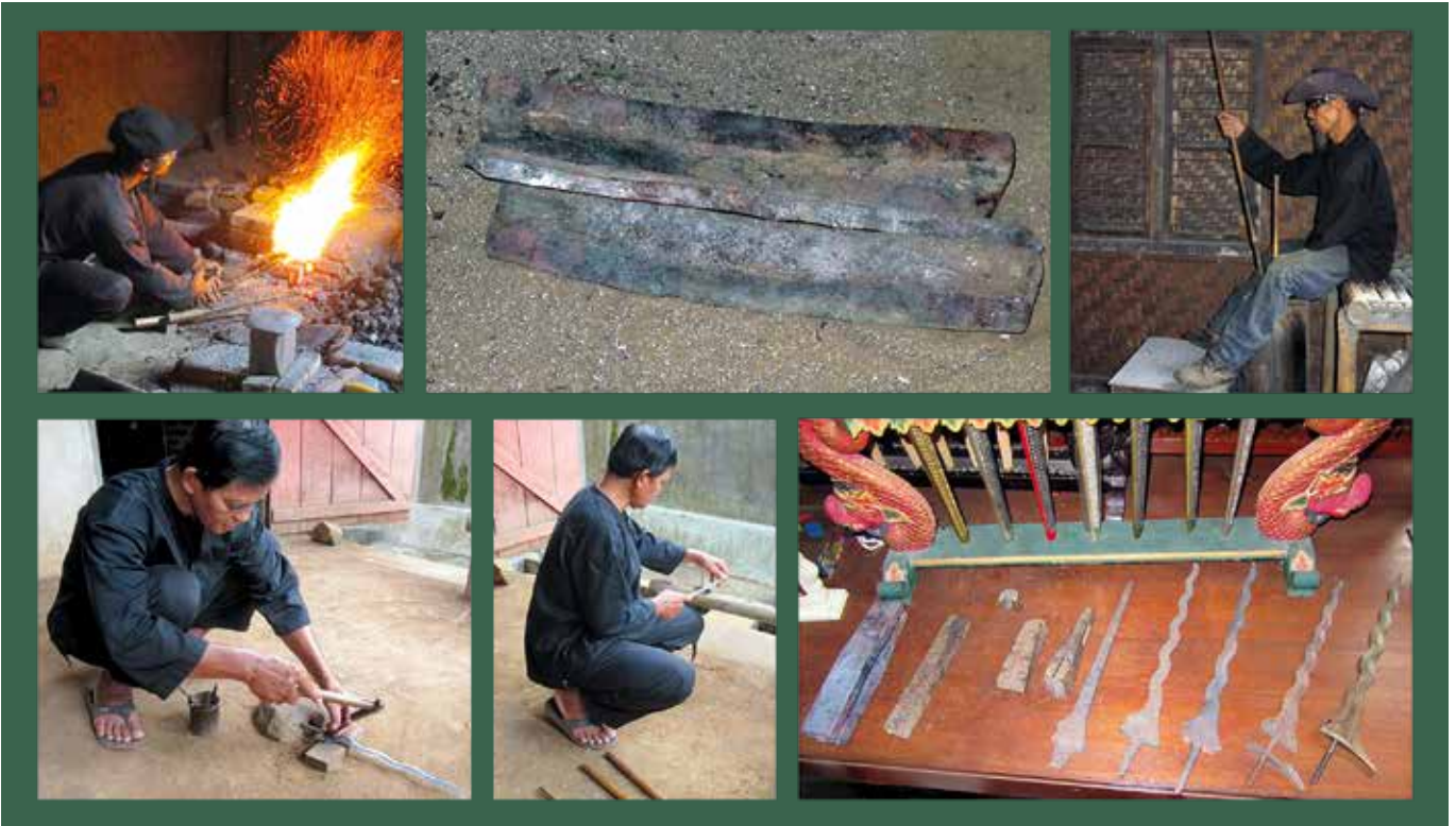
Forging a keris from billet to finished blade. Photos by Darlene Kasten
